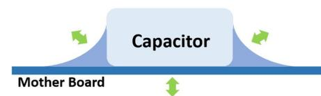
Figure 7. A capacitor exhibits an inverse piezoelectric effect due to the electric field.
